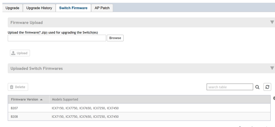
FIGURE 239 Upgrading the Switch Firmware
